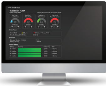
UPS-SolidSwitch Kontrol Paneli
